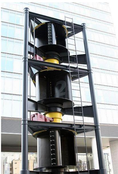
**Fig. 6a&b: Left: A Stacked Savonius turbine, with three blades per sub-turbine. Right: Diagram of wind patterns within a two bladed Savonius turbine.** (Savonius wind turbine, 2009)
